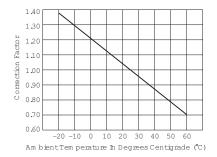
To use this chart: Read up from the ambient temperature to the curve, and across to find a correction factor. Multiply the breaker rating by the correction factor to determine the compensated rating. Calculate the overloads in terms of the compensated rating to use the published trip curve. Do not use these devices outside their specified
